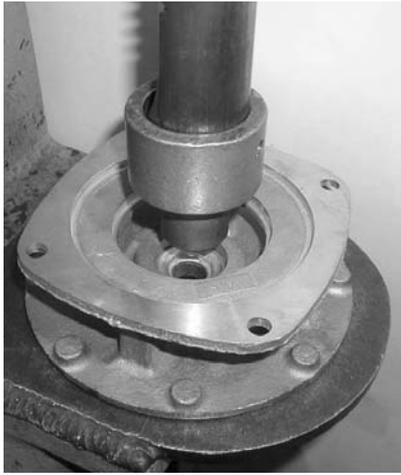
**4. Press Seal from Pump Body or from the Pump Casting Containing the Seal**
